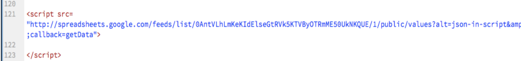
Figure 6 - An excerpt of the code which tells the code to grab my Google Spreadsheet and its information through the command callback=getData.
