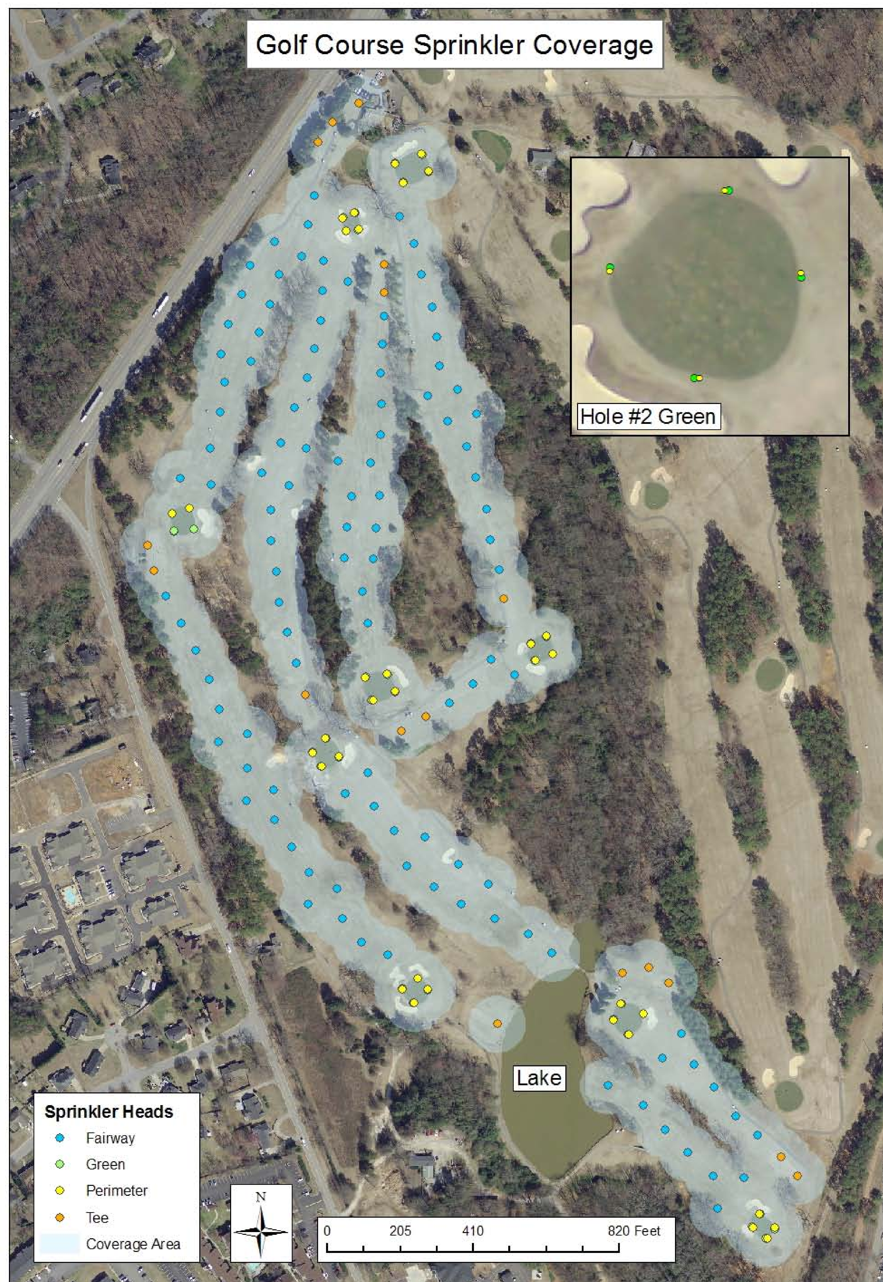
Figure 2. Map of golf course irrigation system with sprinkler heads, water coverage, and inset of Hole #2 Green illustrating Green and Perimeter heads.
