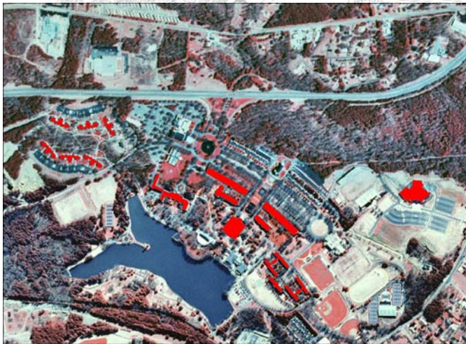
Figure 1. The building footprints (in red) are laid out on top of the orthographic photo.
